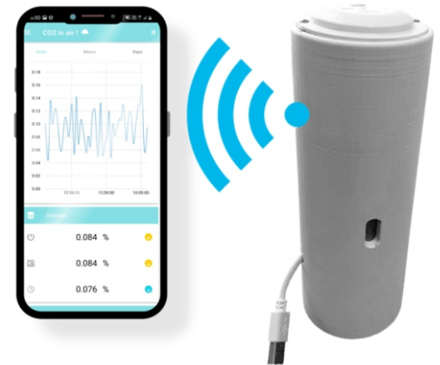
Mobile HMI app and CO 2 sensor with TapNLink
