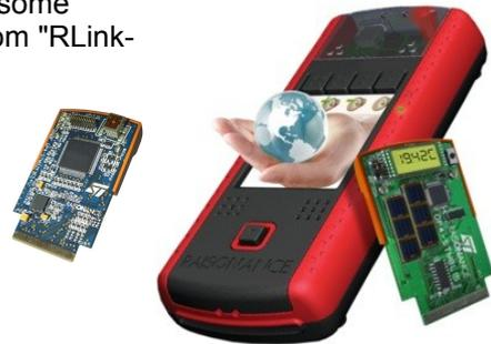
When the **OP4-RLink-ADP** daughterboard is plugged in the **Open4** base, the resulting **Open4-RLink** can be used as a standard RLink, with the same adapters as a Rlink3.xx.
