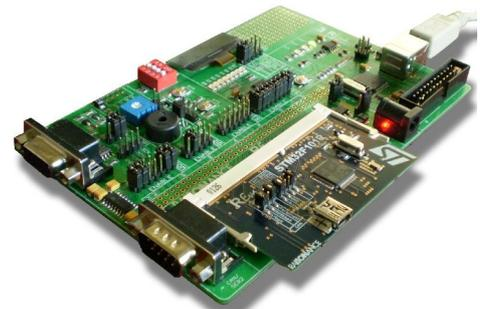
**RLink-STD** provides unlimited debugging of applications on supported 8-bit devices via the same connection while driven from the Ride7 integrated development environment.
