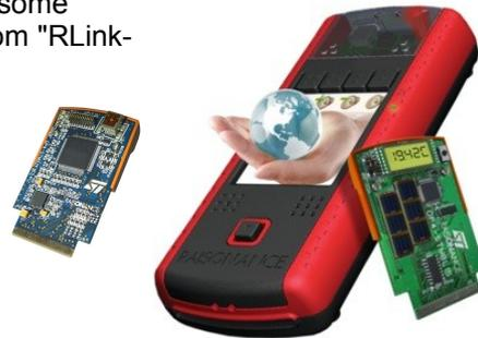
When the **OP4-RLink-ADP** daughterboard is plugged in the **Open4 base**, the resulting **Open4-RLink** can be used as a standalone RLink, with the same adapters as a standalone RLink.
